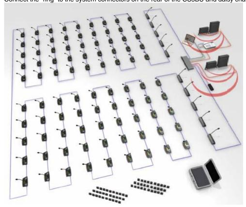
Use no cables that are longer than 330 feet (100 m) to connect one microphone station to another.
